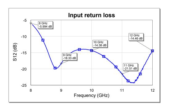
Test fixture data for Bare Die Vd1 = Vd2 = 2 V, Vd3 = 5 V, Total Current = 80 ma, TA = 25 °C
