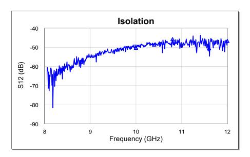
Test fixture data for Bare Die Vd1 = Vd2 = 2 V, Vd3 = 5 V, Frequency = 9.6 GHz Total Current =75 ma, T<sub>A</sub> = 25 °C
