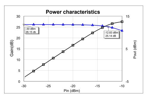
Pout at 1 dB compression @ 9.6 GHz = 12 dBm
